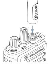
To remove the antenna, turn the antenna counterclockwise.
