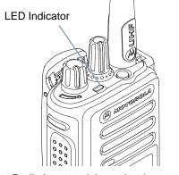
**Blinking red** – Radio is transmitting at low battery condition, receiving an emergency transmission, has failed the self-test upon powering up, or has moved out of range if radio is configured with Auto-Range Transponder System.
