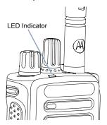
The LED lights up solid green while the radio is transmitting and blinks when the radio is receiving.
