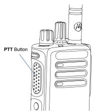
While a call is not in progress, the PTT button is used to make a new call (see Making a Radio Call on page 18).
