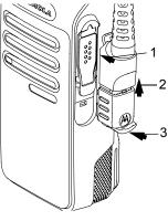
To remove the accessory connector, refer to the steps shown in the diagram.
