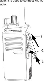
Attaching the Universal Connector Cover (Dust Cover)
