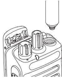
With the radio turned off, set the antenna in its receptacle and turn clockwise.
