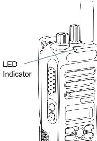
**Blinking yellow** – Radio is scanning for activity or receiving a Call Alert, or all local Linked Capacity Plus channels are busy.
