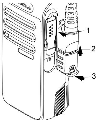
To remove the accessory connector, refer to the steps shown in the diagram.
