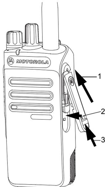
Insert the slanted end of the cover into the slots above the universal connector. Press downwards on the cover to seat the dust cover properly on the Universal Connector.
